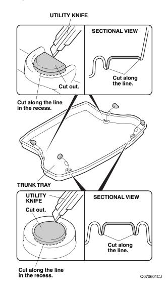
3. Open the trunk lid. Place the trunk tray on the trunk floor
